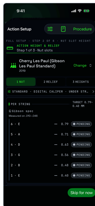
The action setup at the nut step, with the published target for each string.
